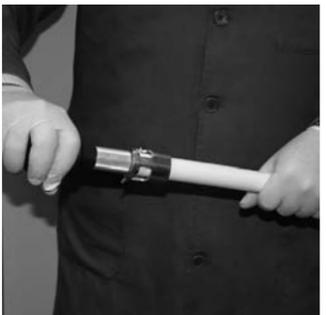
It is mandatory to insert the calibrator / reamer ref. AE inside the tube, turning until filing the inside and outside edge of it. Such operation is essential to facilitate the insertion of the fitting into the tube and prevent the o-rings from being damaged, or displaced from their housing.
