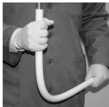
The minimum bending radius specified in the table must always be respected in order to avoid pipe throttling.
