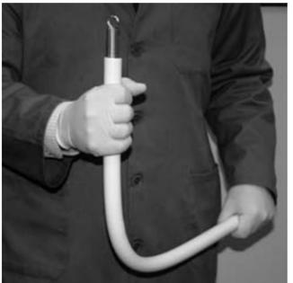
When it comes to getting a very tight curve, it is advisable to use an internal or external spring, adapted to the diameter of the tube that we are going to bend (see page 43).
