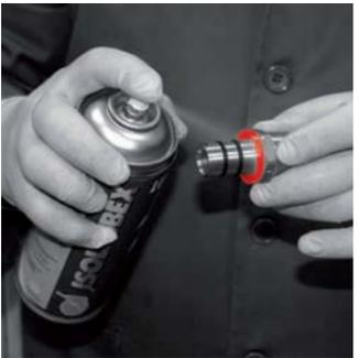
Lubricate the part of the accessory that is inserted.
