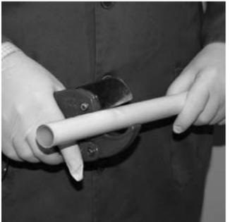
Cut the tube perpendicular to its length, using a tool that guarantees a clean and precise cut.
