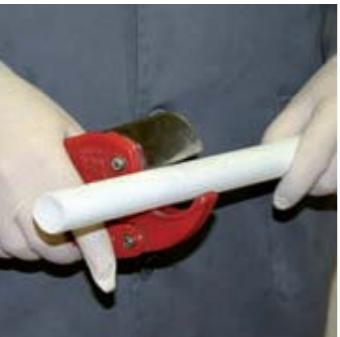
Cut the tube perpendicular to its length, using for it a tool that guarantees a clean and precise cut.
