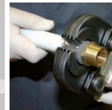
Position the pliers, of the measure corresponding to the tube, in the stainless steel cap, as close as possible to the electrolysis joint.
