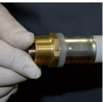
The fitting must be inserted in the tube to its base so that the stainless steel cap is attached to the anti-electrolysis plastic gasket.
