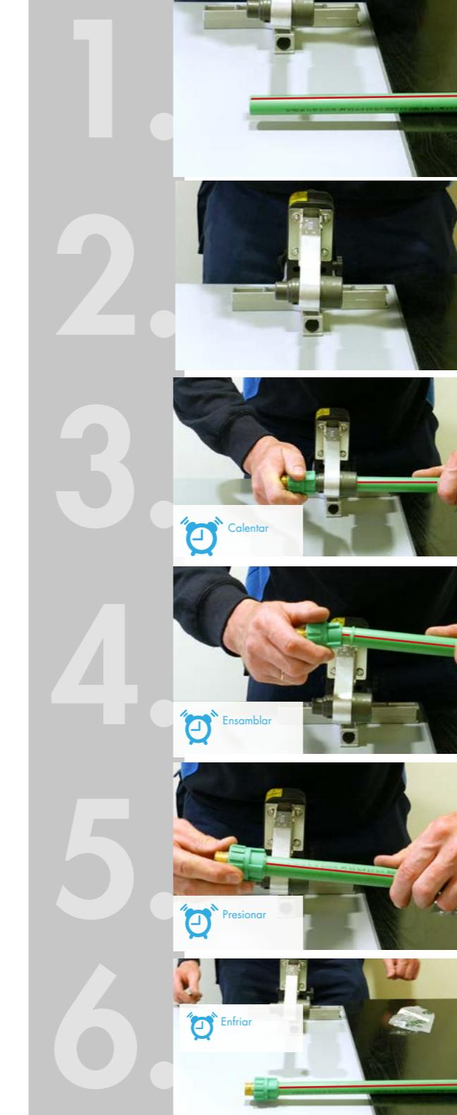
Cut the tube perpendicular to its length, using a tool that guarantees a clean and precise cut.
