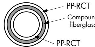
The intermediate layer with the glass fiber composite is fused with the PP-RCT material of the tube wall.
